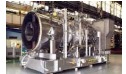
Sources : 1) Antonio Villalba-Herreros et al., Techno-Economic Assessment of Large-Scale Green Hydrogen Logistics Using Ammonia As Hydrogen Carrier: Comparison to Liquefied Hydrogen Distribution and In Situ Production, ACS Sustainable Chem. Eng. 2023, 11, 12, 4716–4726. 2) Mitsubishi's ammonia gas turbine
